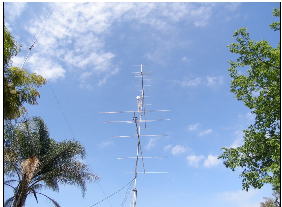
Hans ZR6HVG and Pieter ZS6PA erecting portable 6m and 2m yagis as well as a 1.3 GHz helical
